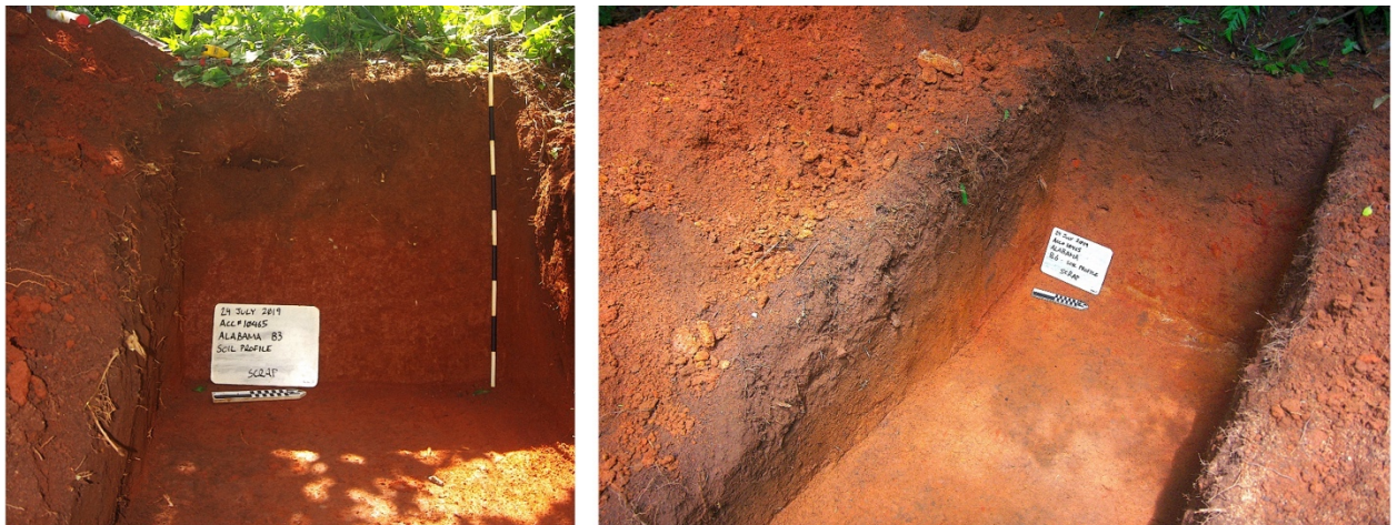
Figure 2.14: Stratigraphic profile in Borrow Pits 3 (left) and 6 (right).
